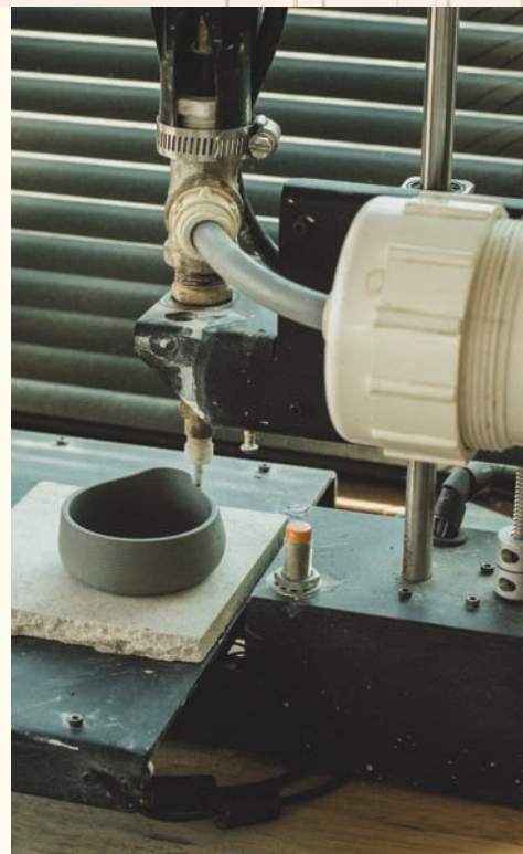
Sutton maps out the design on the computer, transfers it directly to the machine and prints a ceramic mug in about seven minutes.
